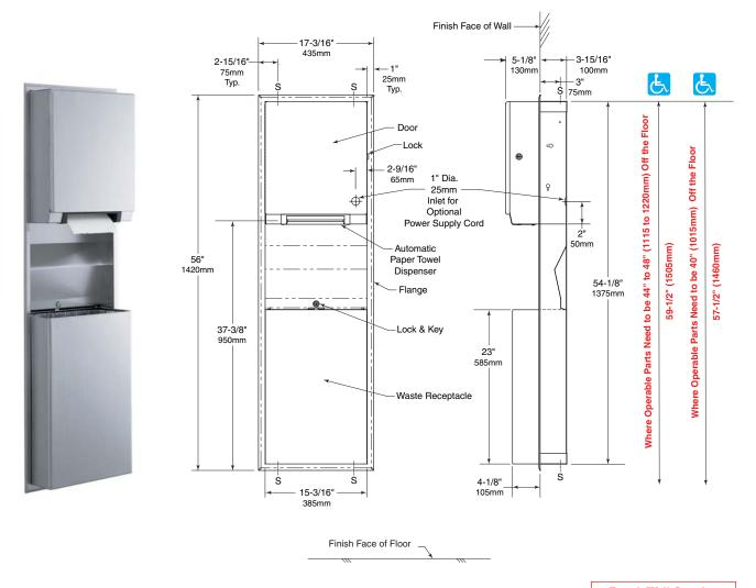
Rough Wall Opening 16" (405mm) wide 54-3/4" (1390mm) high 4" (102mm) minimum recessed depth
